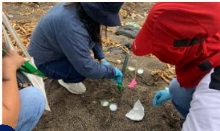
Set up air contamination controls. 2
