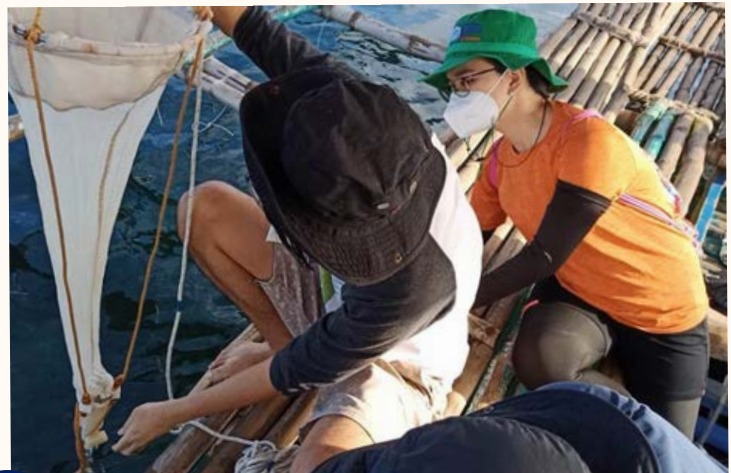
Tow net for 10 minutes and collect sample.
